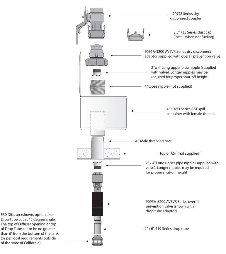
The Drop Tube Diffuser and Overfill Prevention device may have to be removed (if installed) upon District request to verify the existence of a submerged fill pipe.
