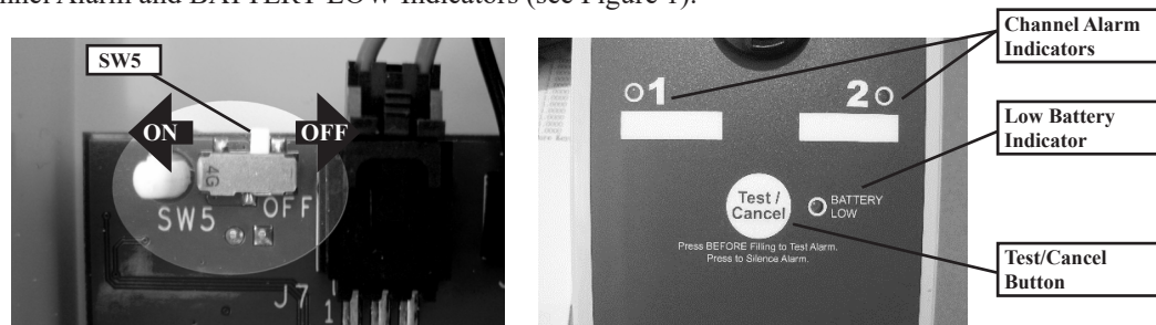
Fig. 1 Power Switch (SW5) ... Channel Alarm Indicators, Battery Low Indicator and Test/Cancel Button on the 918D
