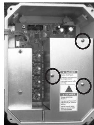
**Figure 8 - Installing the Facilities Cover**
