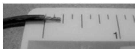
Strip off about  $\frac{1}{4}$  inch (5mm) of insulation from the wire and twist the ends of the wire.
