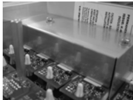
**Figure 5 Installing the I.S. Cover**
