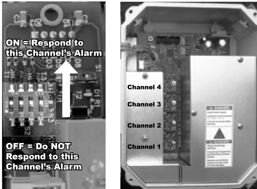
**Figure 8 - Output Module Alarm Channel Configuration**
