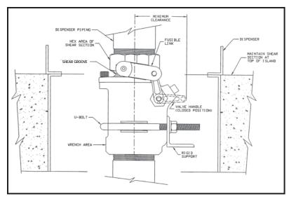
**Warning**: This valve must be rigidly anchored to the island form or dispenser sump valve support brackets to insure breakage at the shear groove in the event of dispenser impact. Failure to provide rigid mounting may result in failure of the valve to shut off in the event of dispenser impact, resulting in a hazardous condition.
