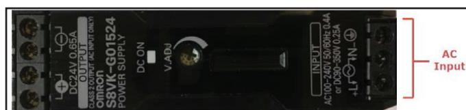
Figure 6—AC Input Connections
